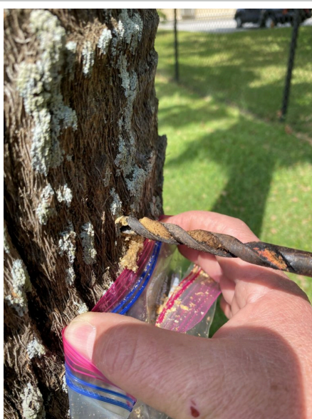
Obtaining a sample for testing using a sterile drill bit.
